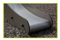
**1- The sliding surface** is made of 2mm thick stainless steel, which is shaped, bent and rolled from one piece.
