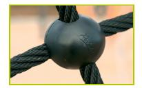
**4- The 16mm diameter ropes** are made of galvanised steel cable covered with polyester. The cables are linked together and held in place by injected polyamide spheres.
