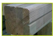
3- The 68mm square posts are made of laminated timber, which have not been treated with chrome or arsenic. Splinter-free, the laminate provides great strength and dimensional stability. The posts are protected from wear and tear caused by fungi and insects.
