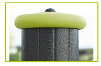
1- The 125mm diameter post is made of painted galvanised steel. The two-tone grey grained finish has a slightly undulating surface for increased scratch resistance. The cap is made of injection moulded polyamide.
