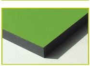
6- The coloured panels are made from a 13mm thick compact material (HPL). Robust in construction, it has excellent weather and vandal resistance properties.
