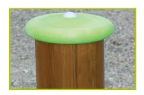
1- The 125mm round post is made of laminated timber, which has not been treated with chrome or arsenic. Splinter-free, the laminate provides great strength and dimensional stability. The post is protected from wear and tear caused by fungi and insects. The cap is made of injection moulded polyamide.
