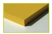
1- The lacquered panels are made from very high quality plywood 22mm thick, made of alternate layers of thin birch, which offers longevity and an exceptional mechanical strangth. The colours are applied by electrostatic spraying of two-component polyurethane lacquer that is free of heavy metals, to ensure high levels of resistance to potentially aggressive chemicals such as anti-graffiti cleaning products.
