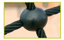
**4- The 16mm diameter ropes** are made of galvanised steel cable covered with polyester. The cables are linked together and held in place by injected polyamide spheres.
