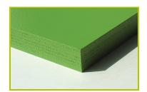
1- The lacquered panels are made from very high quality plywood 22mm thick, made of alternate layers of thin birch, which offers longevity and an exceptional mechanical strangth. The colours are applied by electrostatic spraying of two-component polyurethane lacquer that is free of heavy metals, to ensure high levels of resistance to potentially aggressive chemicals such as anti-graffiti cleaning products.
