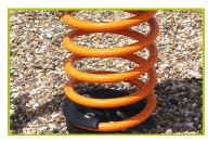
2- The springs are made from Grade 35SCD6 steel, shot blasted, stress relieved, zinc coated and finished with two coats of epoxy polyester powder.
