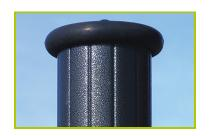
**1- The 125mm diameter post** is made of painted galvanised steel. The two-tone grey grained finish has a slightly undulating surface for increased scratch resistance. The cap is made of injection moulded polyamide.
