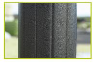
4- The 125mm diameter posts are made of painted galvanised steel. The grained finish has a slightly undulating surface for increased scratch resistance.
