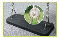
4- The swing seats are made of shock absorbing moulded honeycomb rubber. The swing chains are made of stainless steel. The seat fixing brackets are made of 10mm stainless steel wire. PVC sliding rings are fitted to limit the wear of the metal parts over time. The rings are accessed by a vandal proof, stainless steel shackle.
