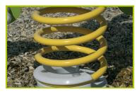
2- The spring is made from Grade 35SCD6 steel, shot blasted, stress relieved, zinc coated and finished with two coats of epoxy polyester powder.
