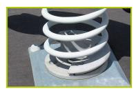
3- The spring is made from Grade 35SCD6 steel, shot blasted, stress relieved, zinc coated and finished with two coats of epoxy polyester powder.
