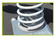
**2- The spring** is made from Grade 35SCD6 steel, shot blasted, stress relieved, zinc coated and finished with two coats of epoxy polyester powder.
