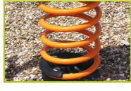
4- The springs are made from Grade 35SCD6 steel, shot blasted, stress relieved, zinc coated and finished with two coats of epoxy polyester powder.
