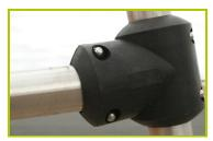
**6- Injection moulded polyamide fixings** connect the posts with the platforms and the various play features. They are non-toxic, flameproof and U.V. resistant. The thickness of the polyamide makes the equipment both strong and vandal resistant.
