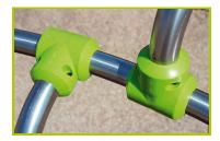
**4- Injection moulded polyamide fixings** connect the posts with the platforms and the various play features. They are non-toxic, flameproof and U.V. resistant. The thickness of the polyamide makes the equipment both strong and vandal resistant.
