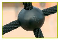
8- The 16mm diameter ropes are made of galvanised steel cable covered with polyester. The cables are linked together and held in place by injected polyamide spheres.
