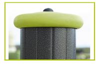
1- The 125mm diameter posts are made of painted galvanised steel. The two-tone grey grained finish has a slightly undulating surface for increased scratch resistance. The caps are made of injection moulded polyamide.
