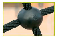
**6- The 16mm diameter ropes** are made of galvanised steel cable covered with polyester. The cables are linked together and held in place by injected polyamide spheres.
