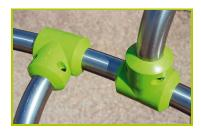
4- Injection moulded polyamide fixings connect the posts with the platforms and the various play features. They are non-toxic, flameproof and U.V. resistant. The thickness of the polyamide makes the equipment both strong and vandal resistant.
