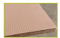
**9- The climbing wall** is made from a 12.5mm thick textured and non-slip compact material (HPL).
