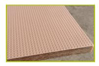
4- The platforms are made from a 12.5mm thick, textured, non-slip compact material (HPL).
