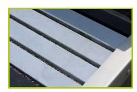
**1- The seat** is a combination of painted steel, 50x25x2.5mm, and pultruded polyester slats (compact polyester / fibre glass) 58x25x3mm, RAL 7004.
