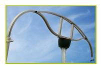
**1-** The supporting arm is made of a 60x60mm stainless steel tube with twin curves. The twin reinforcing struts give the supporting structure its rigidity. The unit as a whole is bolted to the plate on the galvanised steel post (Ø 140mm).
