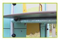
2- The platforms are made from a 12.5mm thick, textured, non-slip compact material (HPL). Further reinforcement is provided by galvanised steel supports, located on the underside of the platforms.
