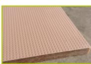
**3-** The steps and the inclined element are made from a 12.5mm thick, textured, non-slip compact material (HPL).
