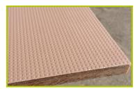
**3- The climbing wall** is made from a 12.5mm thick textured and non-slip compact material (HPL).
