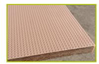
**3-** The steps, the climbing wall and the inclined element are made from a 12.5mm thick, textured, non-slip compact material (HPL).
