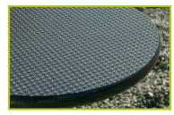
**3- The platforms and the climbing wall** are 21mm plywood panels made up of layers of birch. The surface is coated with a film of non-slip phenolic resin.
