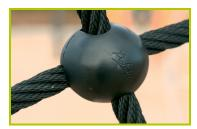
**3- The 16mm diameter ropes** are made of galvanised steel cable covered with polyester. The cables are linked together and held in place by injected polyamide spheres.
