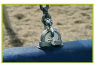
5- PVC sliding rings are fitted to limit the wear of the metal parts over time. The rings are accessed by a vandal proof, stainless steel shackle. The swing chains are made of galvanised steel.
