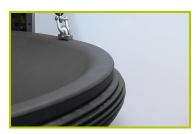
**3- The pod** is made from a single piece of 30%-recycled rotomoulded polyethylene. It is fixed to a stainless steel frame that is fitted with buffers. The pod is suspended from galvanised steel ropes covered by PVC.
