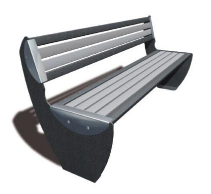
Seat comprises 2 painted steel slats 50x25x2,5 mm, and 4 pultruted polyester slats (polyester composite/fibre glass) 58x25x3 mm, RAL 7004. Seat back comprises 2 painted steel slats 50x25x2,5 mm, and 2 pultruted polyester slats (polyester composite/fibre glass) 58x25x3 mm, RAL 7004. Black polyester powdercoated steel uprights, thickness 8mm - Stainless steel brackets and fixings - Fixing on to a concrete block
