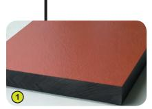
1- The coloured panels are made with a compact material 13mm thick. It is made up of 70% of softwood fibres and 30% of thermosetting resin, and it stands up to weathering very well (sun, rain, damp, etc.). The coloured surfaces are treated with products based on coloured acrylic polyurethane resins; this enables them to stand up well to UV radiation and resist damage.
