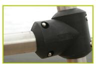
5- Injection moulded polyamide fixings connect the posts with the platforms and the various play features. They are non-toxic, flameproof and U.V. resistant. The thickness of the polyamide makes the equipment both strong and vandal resistant.
