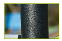
1- The 102mm diameter posts are made of painted galvanised steel. The two-tone grey grained finish has a slightly undulating surface for increased scratch resistance. The caps are made of injection moulded polyamide.
