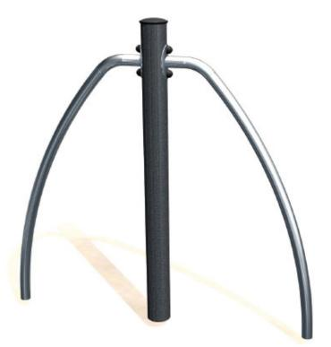
2 stainless steel supports, diameter 40x2mm fixed to a black polyester powdercoated, galvanised steel post, diameter 102m, thickness 2mm, protected by a painted aluminium cap -Stainless steel fixings
