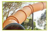
**5- The slide** is made of rotomoulded polyethylene.
