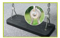
6- The swing seats are made of shock absorbing moulded honeycomb rubber. The swing chains are made of stainless steel. The seat fixing brackets are made of 10mm stainless steel wire. PVC sliding rings are fitted to limit the wear of the metal parts over time. The rings are accessed by a vandal proof, stainless steel shackle.
