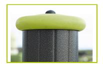
1- The 125mm diameter posts are made of painted galvanised steel. The two-tone grey grained finish has a slightly undulating surface for increased scratch resistance. The caps are made of injection moulded polyamide.
