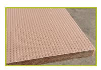
6- The unstable platform is made from a 12.5mm thick textured and non-slip compact material (HPL).
