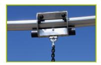
**9- The one-piece rail** is made of stainless steel,  $\emptyset$  76.1mm, 3.6mm thick. The trolley is made of stainless steel ensuring its durability.
