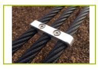
**7- The strap** is made of 3 ropes linked together with aluminium pliers. Each rope, of 16mm diameter, is made up of galvanized steel cables covered in polypropylene.
