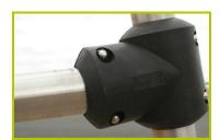
**10-Injection moulded polyamide fixings** connect the posts with the platforms and the various play features. They are non-toxic, flameproof and U.V. resistant. The thickness of the polyamide makes the equipment both strong and vandal resistant.
