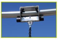
**13-The one-piece rail** is made of stainless steel,  $\emptyset$  76.1mm, 3.6mm thick. The trolley is made of stainless steel ensuring its durability.
