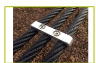
**3- The strap** is made of 3 ropes linked together with aluminium pliers. Each rope, of 16mm diameter, is made up of galvanized steel cables covered in polypropylene.
