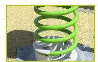
**3- The spring** is made from Grade 35SCD6 steel, shot blasted, stress relieved, zinc coated and finished with two coats of epoxy polyester powder.
