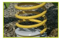
**4- The spring** is made from Grade 35SCD6 steel, shot blasted, stress relieved, zinc coated and finished with two coats of epoxy polyester powder.
