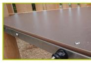
4- The platforms are made from a 12.5mm thick, textured, non-slip compact material (HPL). Further reinforcement is provided by galvanised steel supports, located on the underside of the platforms.
