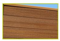
3- The blades are made of wood-plastic composites (WPCs), 95% of which is recycled plastic material (HDPE) and post-industrial wood sawdust. They are covered with a thin decorative brown wooden layer, which makes the material resistant and waterproof, and ensures the colours do not alter over time.
