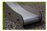
7- The sliding surface is made of 2mm thick stainless steel, which is shaped, bent and rolled from one piece.
