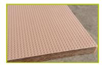
**2- The roof and seats** is made from a 12.5mm thick textured and non-slip compact material (HPL).
